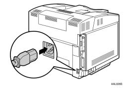
Plug the other end securely into the wall outlet.
