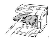
Hold the new toner cartridge and shake it well, about 3 to 4 times, as shown in the illustration
