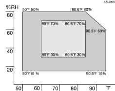
Possible operation range Recommended range The printer must be level within 5 mm, 0.2" both front to rear and
