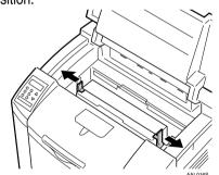
Press the center of the top cover firmly until it locks into position.
