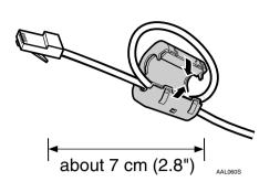
Connect the core end of the Ethernet cable to the connector at the back of the printer and connect the other end to a network device, such as a hub.
